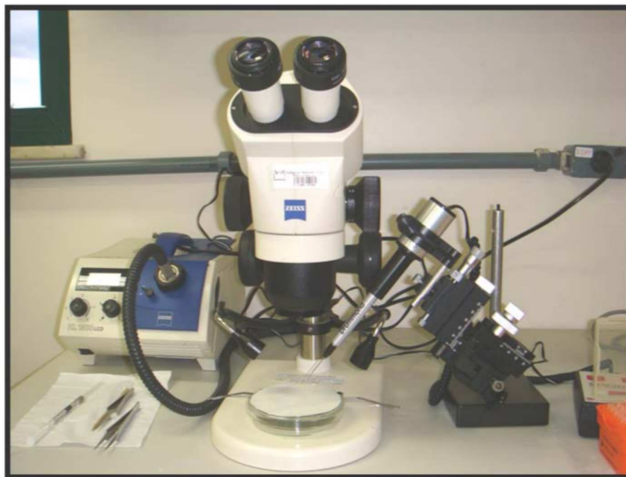
Figura 14: Microinjetor Nanoject II (Drummond)
