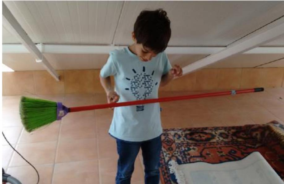
**Figure 1.** Estimated longitudinal position of the CG of a broom, obtained from an unstable static equilibrium technique used to find the CG. The CG is along the vertical line that crosses the wooden stick (the equilibrium is unstable because the CG is above the fulcrum).
