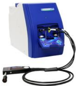
Figura 107 - BWTEK i-Raman Plus portátil.
