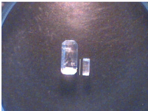
Figure 3. Photographic image showing size comparison: a sucrose crystal seed at the beginning of crystallization and another sucrose crystal seed (with similar initial size and mass) after 72 hours of crystal growth. The vertical white bar is equivalent to 1.74 mm.
