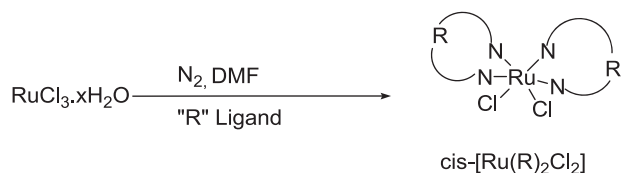
Scheme 4 Synthesis of cis -[Ru(R) 2 Cl 2 ] where R = 1, 10-Phenanthroline/ 2,2'-bipyridyl
