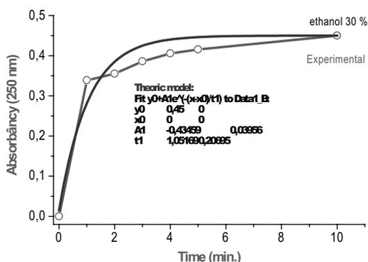
**Figura 3.** Kinetics extraction by ultrasound from *Crotalaria retusa* (experimental) and theoretical model by exponential (first order) with hydroalcoholic solvent 70:30 (H<sub>2</sub>O:EtOH).
