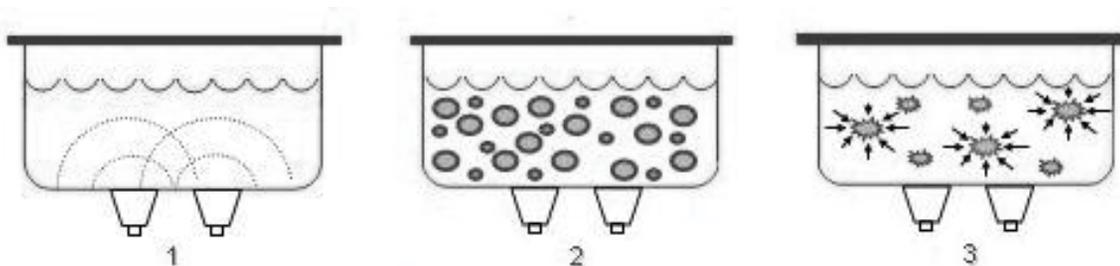
**Figure 2.** Ultrasound scheme. 1) acoustic energy in the ultrasound region; 2) plant cells before the ultrasound radiation; 3) Plant cell suffering the effect of cavitation which leads to its rupture increasing the efficiency of extraction and solubilization in the solvent.
